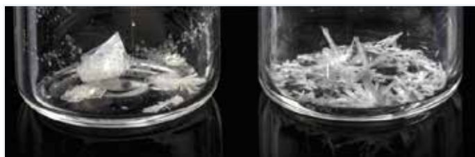
Ibuprofen crystallised from Acetone (left), and Ethyl Acetate, (right)
