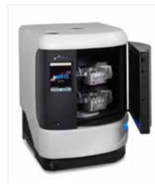
Figure 3. Genevac Series 3 HT evaporator.
