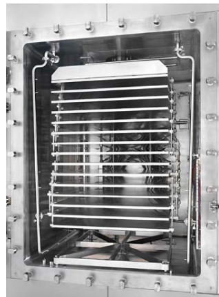
Stoppering Mechanism in a Production Freeze Dryer
