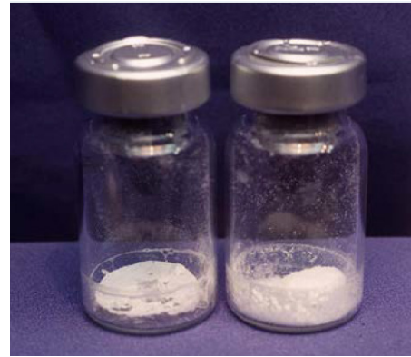
Collapsed Product – Critical Temperature Was Exceeded
