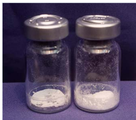
Collapsed Product – Critical Temperature Was Exceeded
