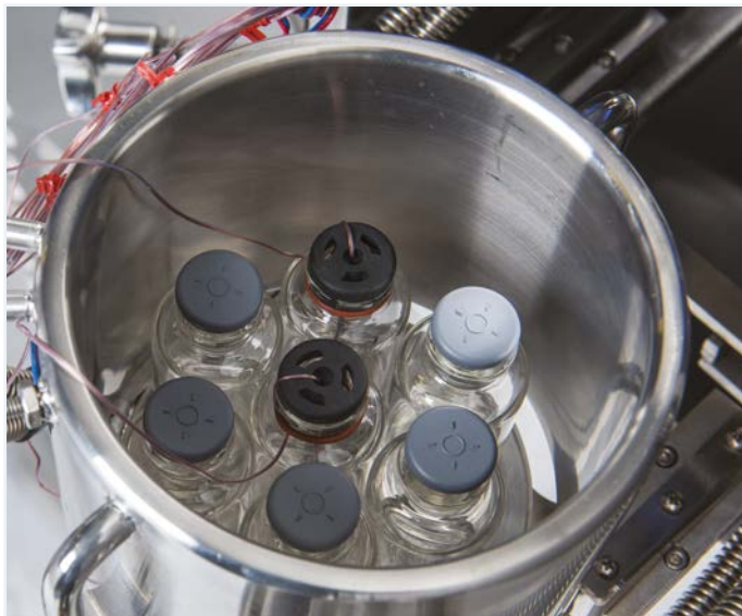
LyoCapsule: 7-vial development freeze dryer
