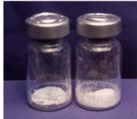
Collapsed Product – Critical Temperature Was Exceeded
