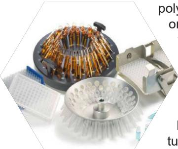
Rotors are available for all common tubes, vials, centrifuge tubes and microcentrifuge tubes. For microtitre plates, two and four place swing rotors will accept multiple plates through the use of stackers. A miVac Duo can hold six shallow plates and the larger miVac 2 Quattro up to twenty shallow-well microplates or eight deep-well plates.
