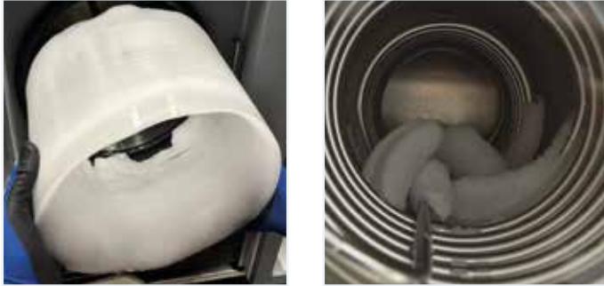
Figure 2. Smooth-wall condenser removal of ice after defrost (left) Internal coil condenser defrost of ice from around coils (right)
