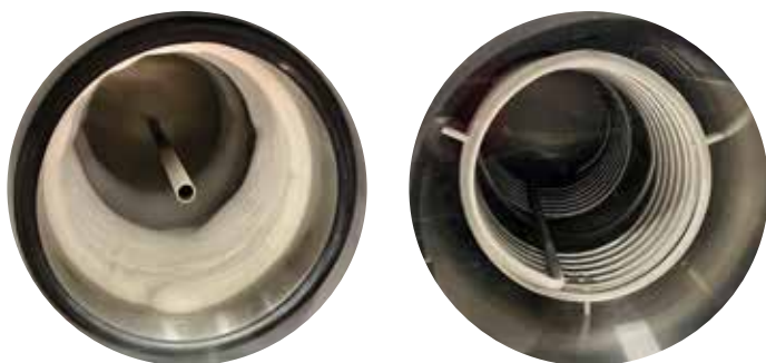
Figure 1. (Left) Smooth-Wall Condenser, (Right) Internal Coil Condenser
