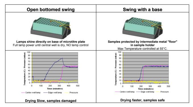
The same principle applies to any sample holder where the light can shine directly onto something other than the base of the swing. For example, years ago it was considered appropriate to have a tube holder, which was a quite open, rack and which exposed the base of each tube to the IR lamp heat.
