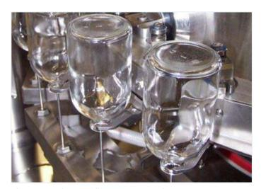
**Figure 1** Washing needles penetrating vials
