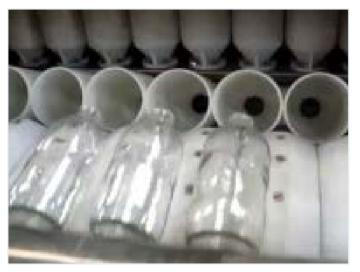
Figure 2: Loading linear washer buckets with vials
