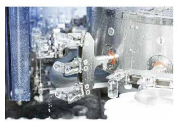
Figure 2: Modern washing and depyrogenation installation featuring washing needles
