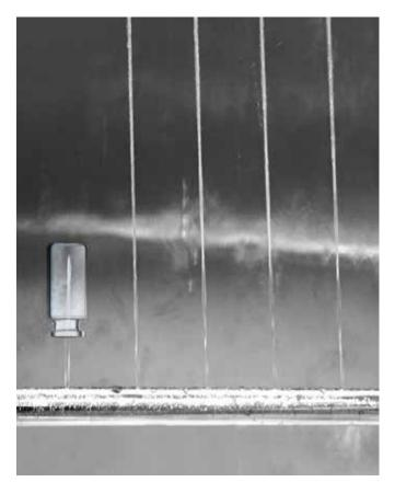
Figure 3: High Pressure Washing Jet Manifold for Vial Washing Without Needles
