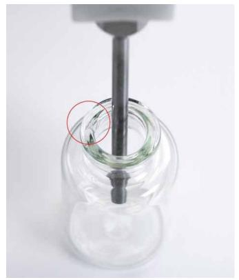
*Figure 1: Chipped vial rim and resultant particulate generation*
