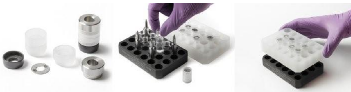
Figure 2. Left to Right: Exalt baffles & tower assembly – Loading vials & towers – Complete holder assembly
