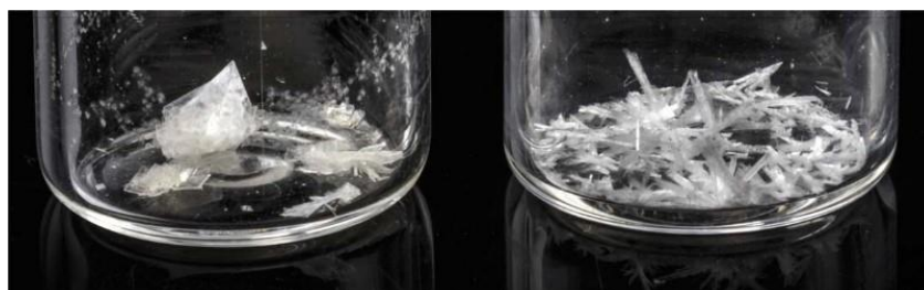
Ibuprofen crystallised from Acetone (left), and Ethyl Acetate, (right)
